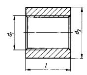
Designation of a welded, black socket of nominal size 40, with R 1 1/2 pipe thread:
